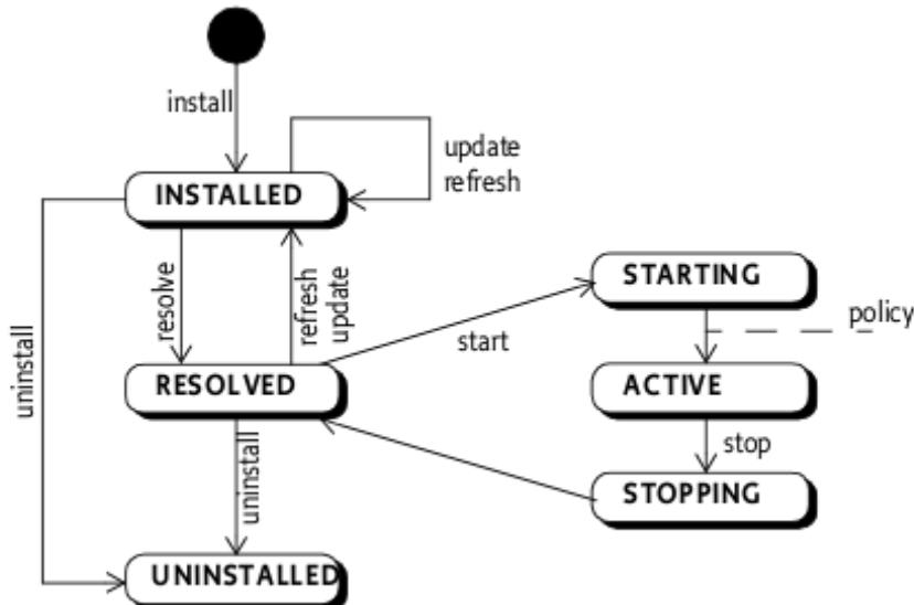
A bundle is activated by calling its **Bundle Activator** object, if one exists. The BundleActivator interface defines methods that the Framework invokes when it starts and stops the bundle.
