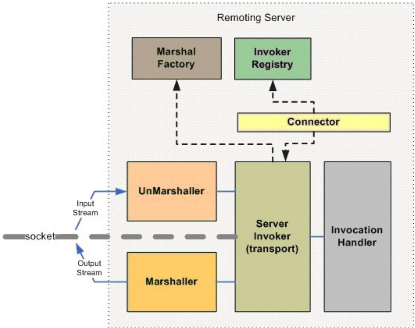
On the server side, it is the Connector class that is used as the external point for configuration and control of the remoting server. The Connector class will call on the InvokerRegistry with its locator to create a server invoker. Once the server invoker is returned, the Connector will then register the invocation handlers on it. The server invoker will use the MarshalFactory to obtain the proper marshal instances as is done on the client side.
