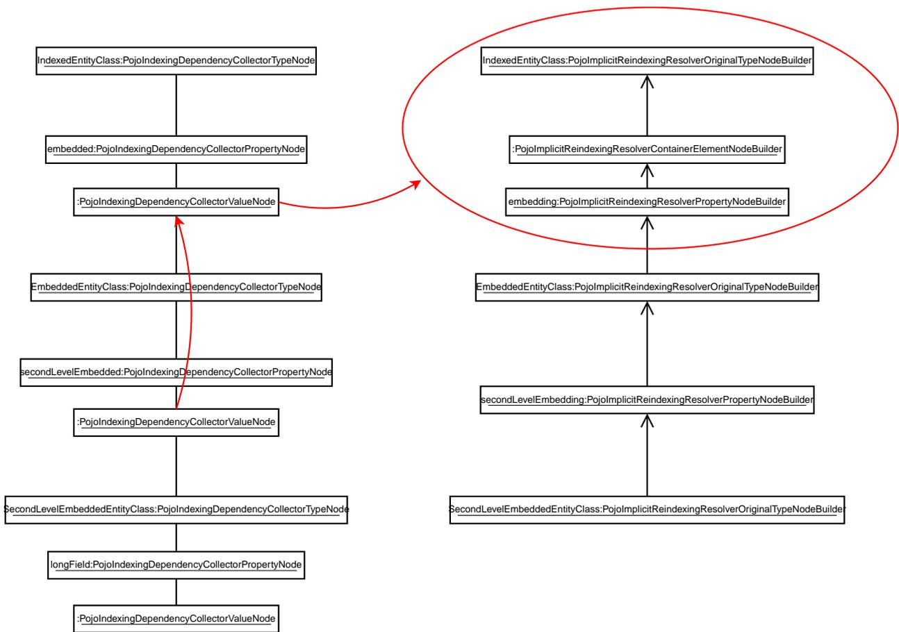
Once we reach the dependency collector root, we are almost done. The reindexing resolver builder tree has been populated with every node needed to reindex `IndexedEntityClass` whenever a change occurs in the `longField` property of `SecondLevelEmbeddedEntityClass`.
