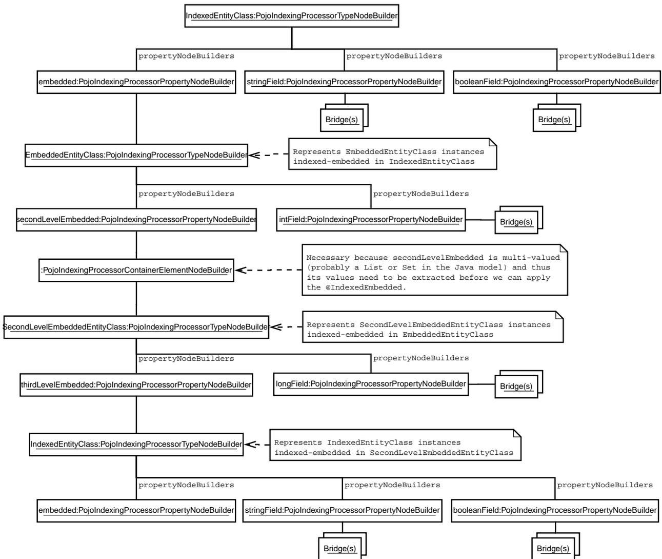
As we build the indexing processors, we will also build another tree to represent dependencies from the root type (`IndexedEntityClass`) to each dependency. This is where dependency collectors come into play.
