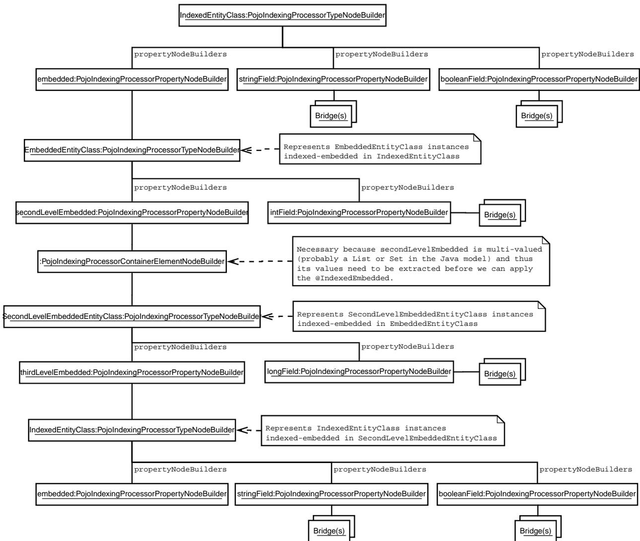
While the mapped model was originally organized as a cyclic graph, the indexing processor nodes are organized as a tree, which means among others it is acyclic. This is necessary to be able to process entities in a straightforward way at runtime, without relying on complex logic, mutable states or metadata lookups.
