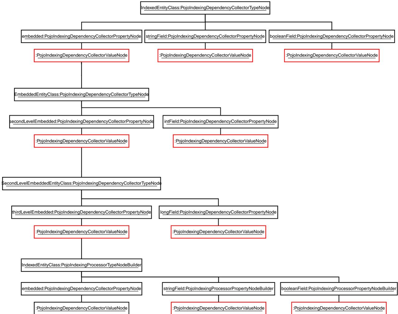
The value nodes in red are those that we will mark as a dependency using `PojoIndexingDependencyCollectorValueNode#collectDependency`. The `embedded` property at the bottom will be detected as not being used during indexing, so the corresponding value node will not be marked as a dependency, but all the other value nodes will.
