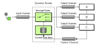
In **Camel 2.5** we introduced a dynamicRouter in the DSL which is like a dynamic Routing Slip which evaluates the slip *on-the-fly*.
