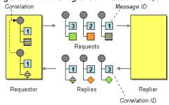
The use of a Correlation Identifier is key to working with the Camel Business Activity Monitoring Framework and can also be highly useful when testing with simulation or canned data such as with the Mock testing framework
