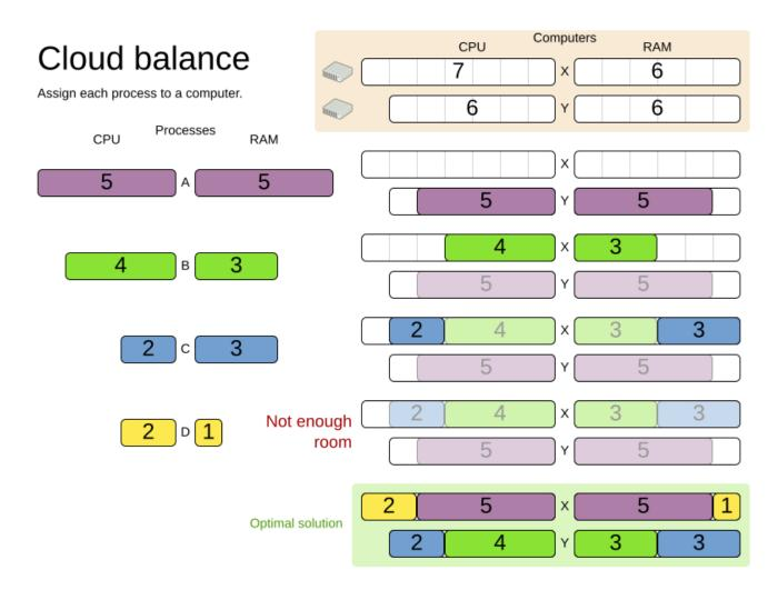
The simple algorithm used here is the *First Fit Decreasing* algorithm, which assigns the bigger processes first and assigns the smaller processes to the remaining space. As you can see, it is not optimal, as it does not leave enough room to assign the yellow process D.
