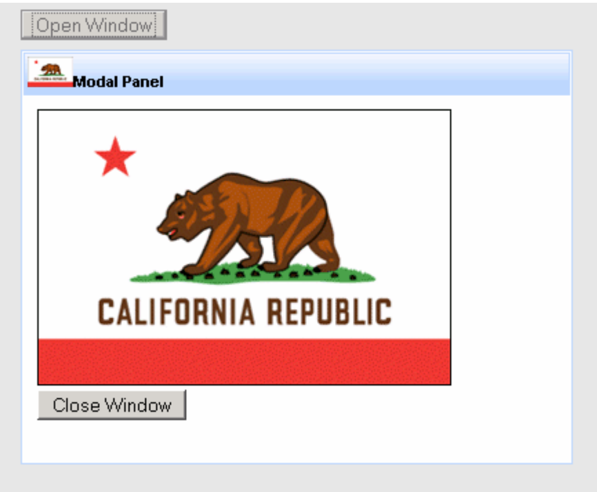
Figure 6.193. The <rich:modalPanel> component opens in closest to observer layer. All other layers are dimmed by blocking <div> element (gray on the picture).
