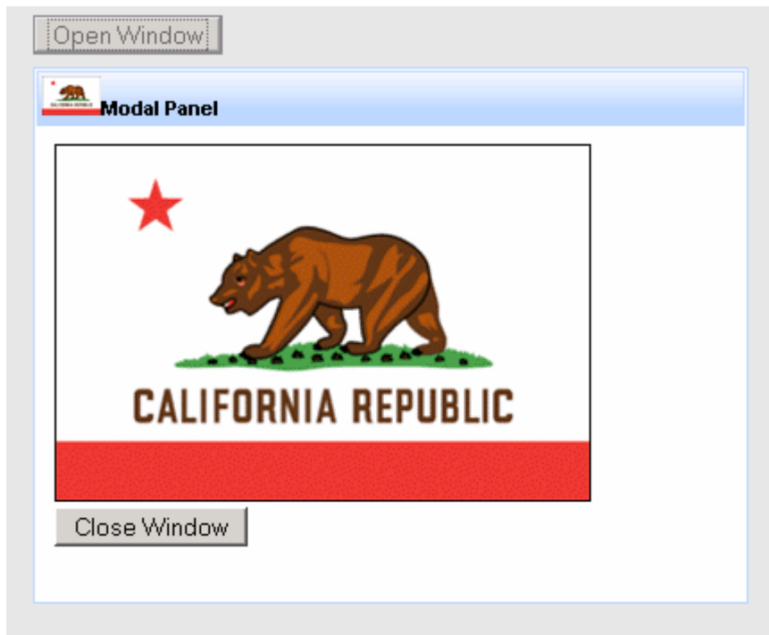
Figure 6.199. The <rich:modalPanel> component opens in closest to observer layer. All other layers are dimmed by blocking <div> element (gray on the picture).
